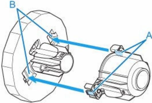
5. Insert holder stopper from left into roll holder as shown, and then while holding in position (B), push firmly until holder stopper flange (A) touches roll paper. Lock the holder stopper lever (C) by rotating it towards
