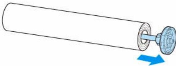
3. To remove 3-Inch Paper Core Attachment, press tabs (A) inward and remove attachment.
