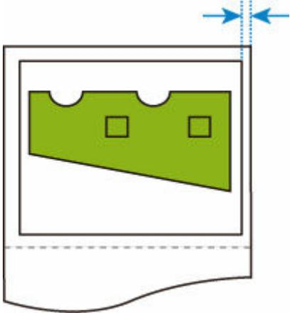
If the lower roll of paper has smaller margins than the upper roll of paper, from which the paper has been fed, then paper is switched automatically, and the image is printed on the lower roll paper.
