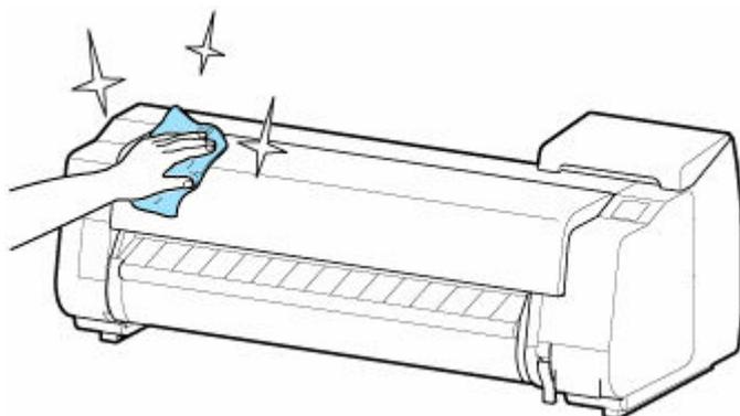
Open the top cover and output guide and clean parts that come in contact with paper (A, B), sensor (C) and window on the back side of the top cover.
