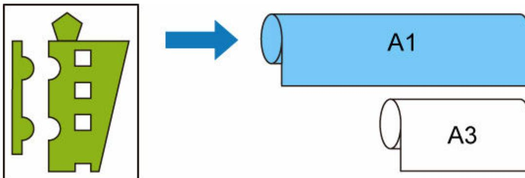
When the A1 width roll paper is loaded on the upper roll, A3 width roll paper on the lower, and the paper source can be switched, and when an A4 size image is enlarged by 160 % specified in **Scaling** on **Enlarge/Reduce**, the A1 width roll paper is selected, as the image width exceeds that of A3.
