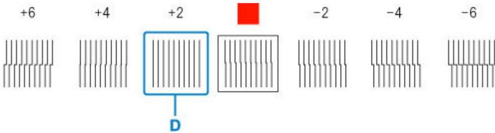
Example 2: Move the angle adjustment lever to a position between the numbers or between the number and the square (E) of the two sets of lines that are least misaligned. In this case, select -1.
