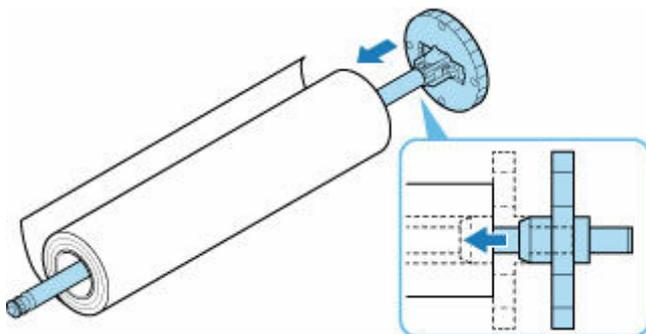
3. Load roll paper in printer or roll unit. (See "[Loading the Upper Roll on the Printer.](#)") (See "[Loading the Lower Roll on the Roll Unit \(Option\).](#)")
