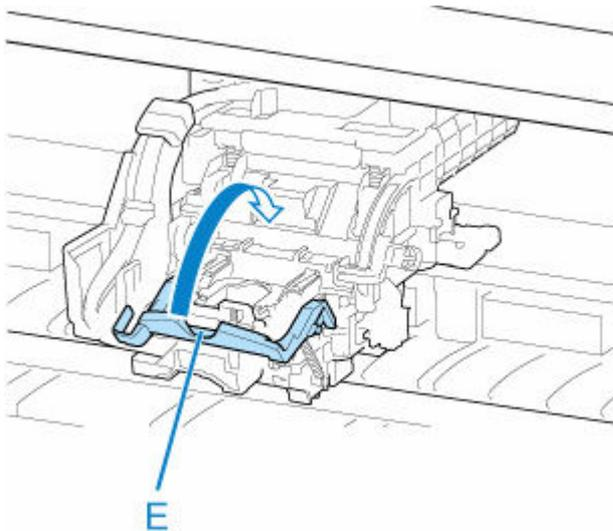
**17.** Adjust angle adjustment lever to the position of the red square.
