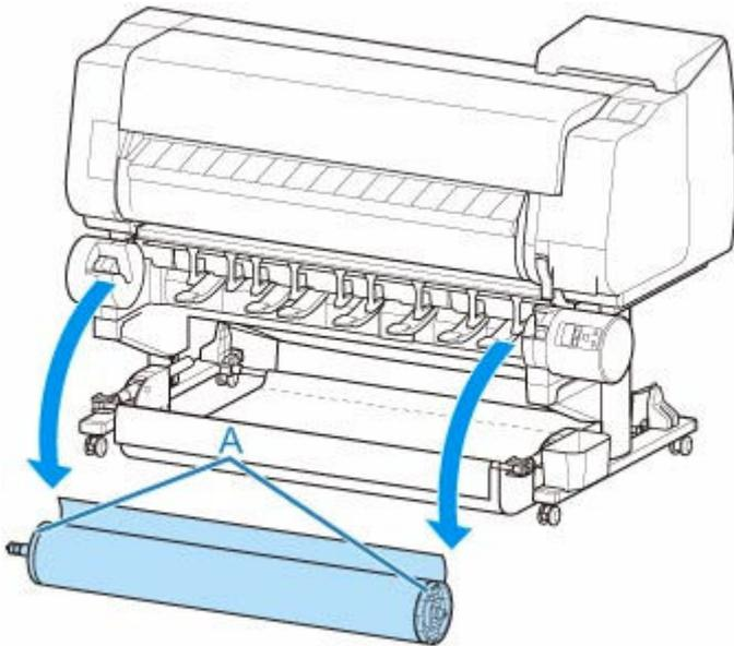
10. Rotate the holder stopper lever (A) towards
