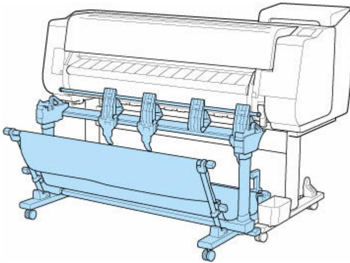
5. If using basket, refer to Printer Stand Setup Guide and attach basket to Stand.
