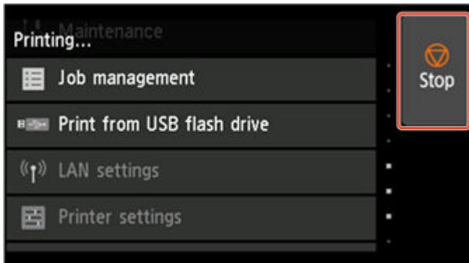
When you press the **Stop** button during printing, the printer operation varies depending on the current status.
