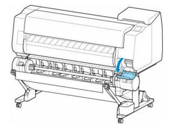
**6.** Hold the used maintenance cartridge by the grip (B) with one hand and put your other hand under the maintenance cartridge to hold it firmly on the bottom, keeping it level as you pull it out.
