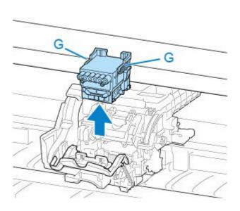
• Never touch the metal contacts of the carriage. Furthermore, do not allow any dirt or debris to become adhered to the metal contacts of the carriage. These may damage the printer.
