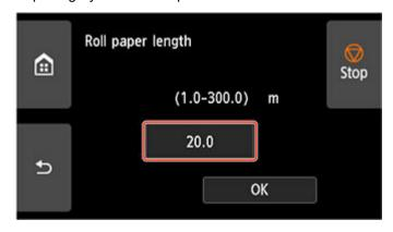
**2.** Tap the keypad appearing on the touch screen, enter the roll paper length, and then tap **OK**.
