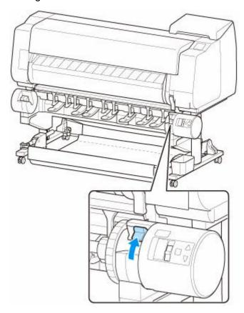
**7.** Hold flanges (A) so that holder stopper is on left, align roll holder shaft with roll holder slot left and right guide grooves (B), and load.
