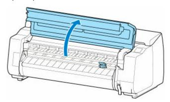
**5.** If cutter blade is dirty, use damp cloth that you have wrung out completely to wipe it clean.
