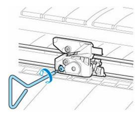
7. Remove cutter blade while holding D.
