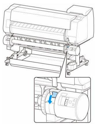
**9.** Change the feed flap switch on top of the roll unit so that the switch indicator (A) is aligned with ● (B) position on the take-up icon.
