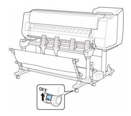
**2.** Pull out the stacker toward you to remove the stacker from the printer.
