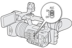
Available values will depend on the gamma curve component of the [Gamma/Color space] setting in the custom picture file. [Wide DR], [Canon Log 3] or [Canon 709]: ISO 500 to ISO 12800 (-2.0 dB to 21.0 dB). [PQ] or [HLG]: ISO 320 to ISO 12800 (-6.0 dB to 21.0 dB).
