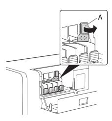
2. Move the lock lever (A) in the direction of the arrow.
