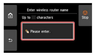
**4.** Enter the wireless router name (SSID). Text entry is case-sensitive.
