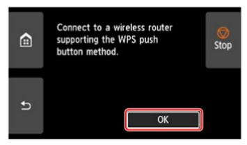
3. Press and hold the WPS button on the wireless router.
