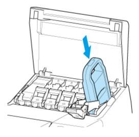
• An ink tank cannot be loaded in the holder if the color or orientation is incorrect.
