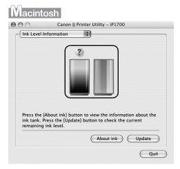
If you install the FINE Cartridge that was once empty and start printing, "?" on the FINE Cartridge appears. Then the following message appears and printing stops. In this case, a remaining level of ink cannot be counted correctly.
