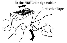
(1) Unpack a new FINE Cartridge and remove the Protective Tape gently.
