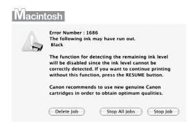
Pressing the **RESUME/CANCEL** button cancels the error indication and enables continuation of printing. However, error detection function is disabled after the error indication is canceled, therefore, **Low Ink Warning** message does not appear later on. When you install new FINE Cartridge, Low Ink Warning is enabled automatically.
