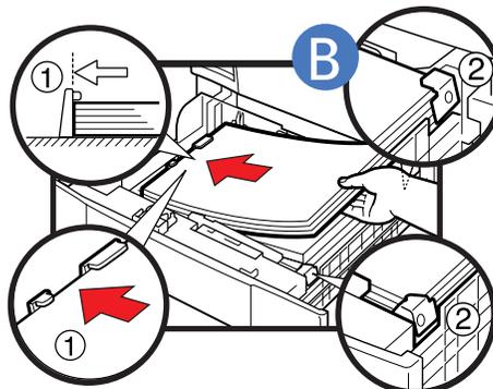
Load the paper stack beneath the cassette's length guide **(1)** and width guide's claws **(2)**.
