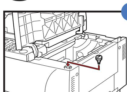
**F** Insert the removed shipping attachment from STEP A into the holder. Keeping the cartridge cover open, go to section 2 - INSTALL CARTRIDGE.
