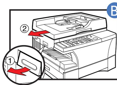
**B** Lift the platen unit lever (1) and slide the platen unit to the left (2).
