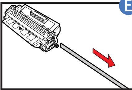
**E** Remove the sealing tape completely.
