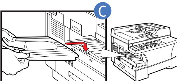
Hook the tab on the output tray onto the opening on the left side of the machine.
