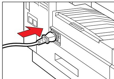
Connect the supplied power cord to the power cord connector on the left side of the machine.
