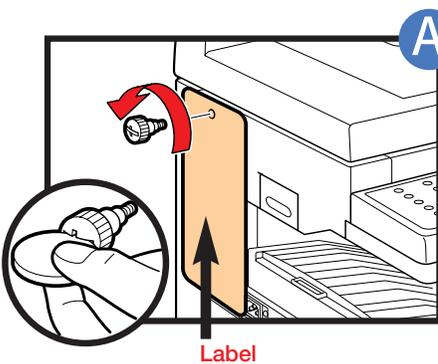
**A** Remove the shipping attachment on the left side using a coin.
