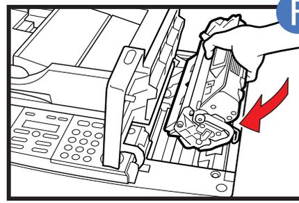
**F** Position the arrow mark on the cartridge towards the inside of the machine, and gently slide the cartridge into the machine as far as it will go.
