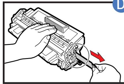
**D** Grasp the cartridge with one hand, firmly and slowly pull out the sealing tape tab with the other hand.
