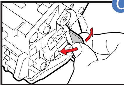
**C** Place the cartridge on a flat and stable surface, grip the sealing tape tab and snap in the direction shown. Make sure that the tab is detached from the cartridge.
