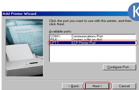
**K** Select the printer port, the machine is connected to (usually LPT1:), then click NEXT. Add Printer Wizard dialog box (Printer name) appears.
