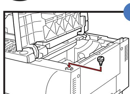
**F** Insert the removed shipping attachment from STEP A into the holder. Keeping the cartridge cover open, go to section 2 - INSTALL CARTRIDGE.
