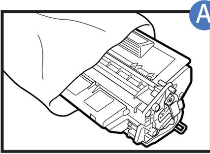
**A** Remove the cartridge from its bag.
