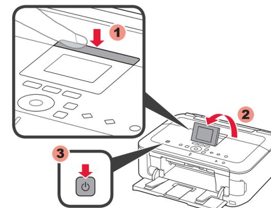
5 Adjust the angle of the LCD, then press the ON button.
