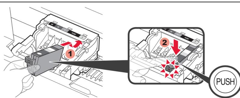
4 Insert and push down the ink tank into the matching color slot.
