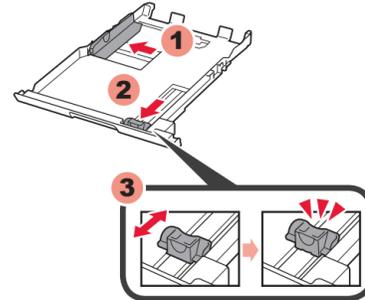
2 Slide the Paper Guide to the sides, then adjust the front guide to the paper size.
