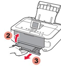
1 When this screen is displayed, close the Output Tray Extension and the Paper Output Tray. Then, pull out the Cassette.
