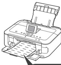
6 In about 6 minutes, the blue-black pattern is printed. Print Head Alignment is complete.
