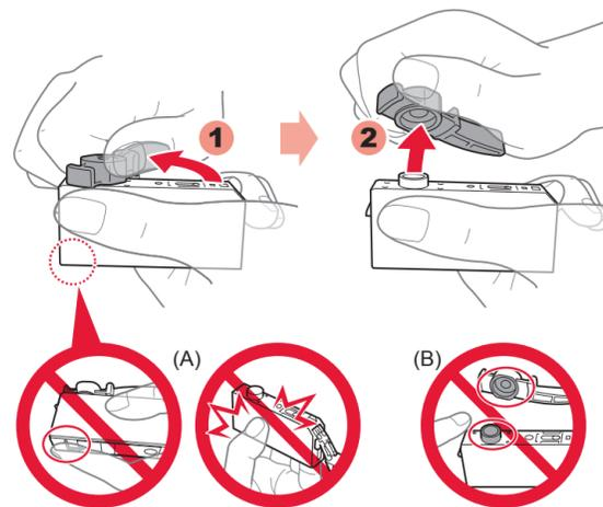
3 Twist and remove the orange cap.
