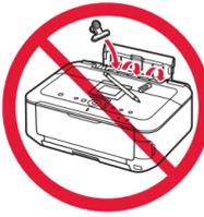
• Do not allow objects to fall inside the machine. These could cause malfunction.
