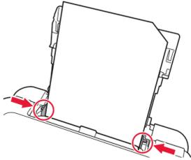
4 Adjust the Paper Guide to fit the paper width.
