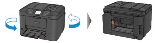
2. If the protective material for the rear cover remains attached, remove it.
