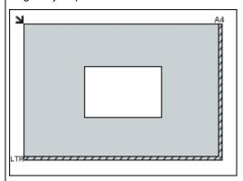
upper corner of the item with the corner at the arrow (alignment mark) of the platen. Portions placed on the diagonally striped area cannot be scanned.
