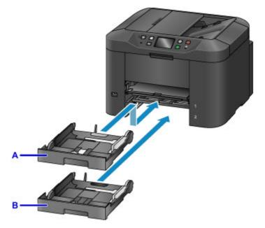
In the upper cassette 1 (A), all sizes of paper compatible with this machine (plain paper, photo paper, envelopes, etc.) can be loaded.
