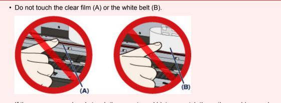
If the paper or your hands touch these parts and blot or scratch them, the machine can be damaged.
