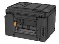
2. If the protective material for the rear cover remains attached, remove it.
