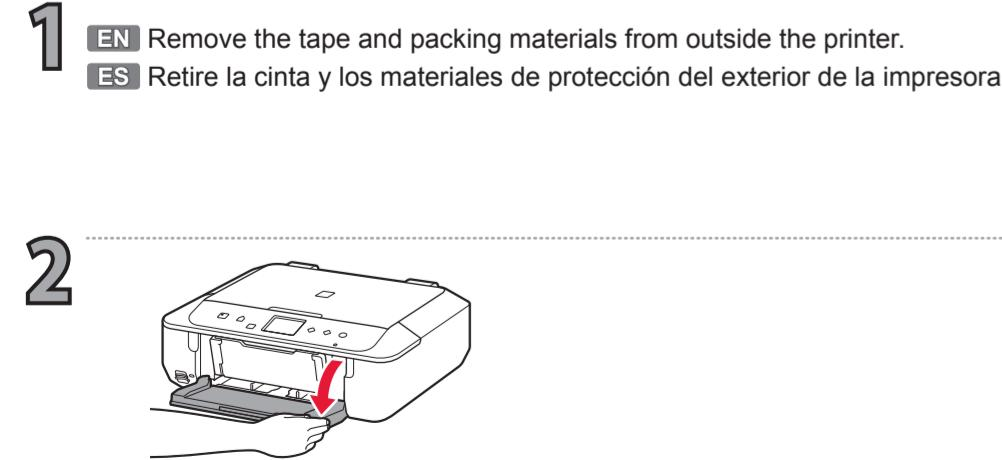
**1** EN Remove the tape and packing materials from outside the printer.
