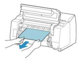
6. If you cannot see the paper, lift the output guide, remove the roll holder, and remove the jammed paper from underneath.
