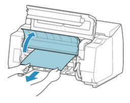
After removing the paper, inspect the interior to ensure paper fragments or other objects do not remain, and lower the output guide.
