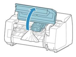
3. If the Carriage is out, move the Carriage out of the way, away from the paper.
