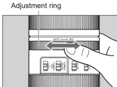
You can adjust the operational feeling (weight of movement) of the zoom ring to a preferred level. Turn the adjustment ring toward SMOOTH to lighten the feeling, and toward TIGHT to strengthen it.
