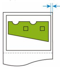
If the lower roll of paper has smaller margins than the upper roll of paper, from which the paper has been fed, then paper is switched automatically, and the image is printed on the lower roll paper.
