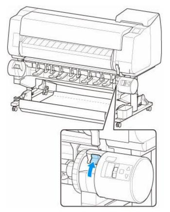
**7.** Hold flanges (A) so that holder stopper is on left, align roll holder shaft with roll holder slot left and right guide grooves (B), and load.
