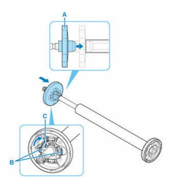
6. Change Roll Holder Lock switch on roll unit to release direction.
