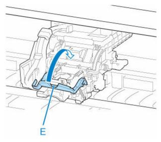
**17.** Adjust angle adjustment lever to the position of the red square.
