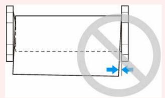
• Depending on the paper, the roll paper may be scratched when being fed and not feed well. In this case, you must feed the paper manually after setting **Paper retention settings** to **Release** on the touch screen. Lift the release lever, advance the roll paper until its leading edge appears on platen, lower the release lever, and then proceed to the next step. However, if **Paper retention settings** is set to **Release**, automatic switching of the upper and lower rolls is not possible.
