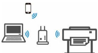
• Without Using Wi-Fi Router (Wireless Direct)
