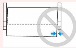
• Depending on the paper, the roll paper may be scratched when being fed and not feed well. In this case, you must feed the paper manually after setting **Paper retention settings** to **Release** on the touch screen. Lift the release lever, advance the roll paper until its leading edge appears on platen, lower the release lever, and then proceed to the next step. However, if **Paper retention settings** is set to **Release**, automatic switching of the upper and lower rolls is not possible.
