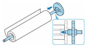
**3.** Load roll paper in printer or roll unit. (See "Loading the Upper Roll on the Printer.") (See "Loading the Lower Roll on the Roll Unit (Option).")
