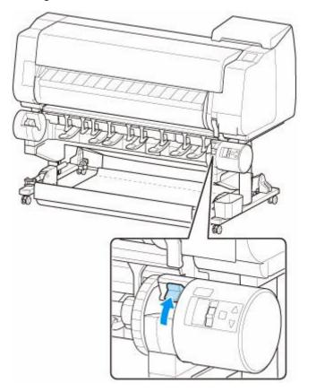
**3.** Hold flanges (A) so that holder stopper is on left, align roll holder shaft with roll holder slot left and right guide grooves (B), and load.
