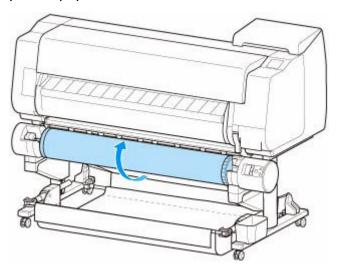
Apply adhesive tape to the rewound paper to hold it in place, if necessary.
