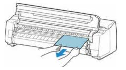
After removing the paper, inspect the interior to ensure paper fragments or other objects do not remain.
