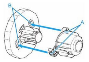
5. Insert holder stopper from left into roll holder as shown, and then while holding in position (B), push firmly until holder stopper flange (A) touches roll paper. Lock the holder stopper lever (C) by rotating it towards .
