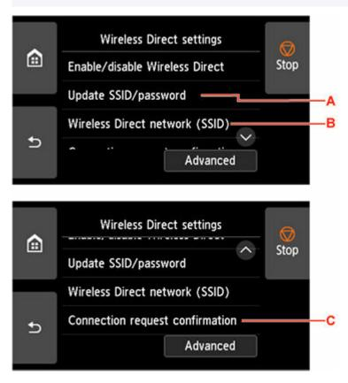
• To update the identifier (SSID) and the password for wireless direct
