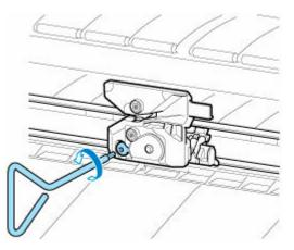
7. Remove cutter blade while holding D.
