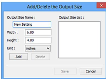
In the **Add/Delete the Output Size** dialog box, multiple output sizes can be specified and then saved at one time. Saved items will be registered to the **Output Size** list and can be selected, along with the predefined items.
