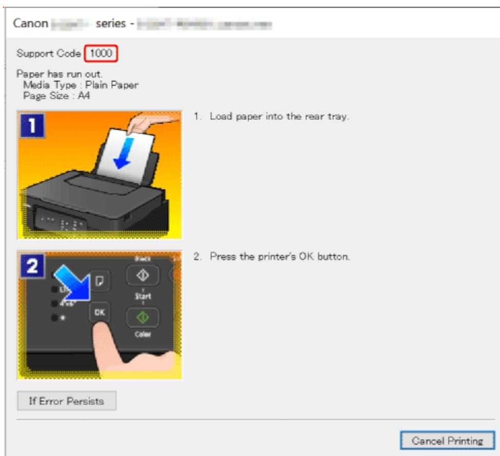
For details on how to resolve errors with Support Codes, see [List of Support Codes for Printer Errors](#).
