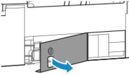
5. Pull out the maintenance cartridge until it stops.
