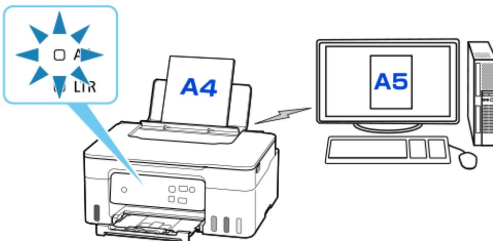
When you start printing, the **Alarm** lamp and the **Paper** lamp for the paper size set when printing will flash.
