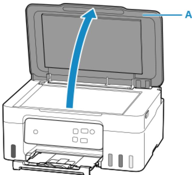
2. Load original WITH THE SIDE TO SCAN FACING DOWN on platen.
