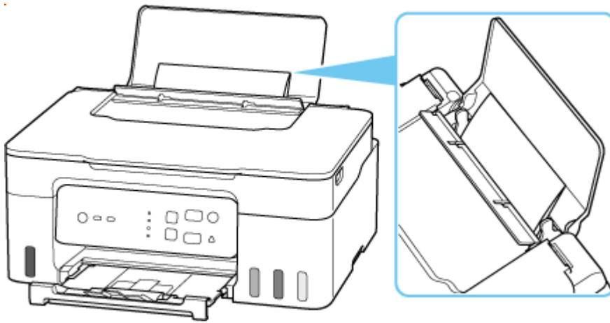
3. Remove foreign object by hand with paper inserted.
