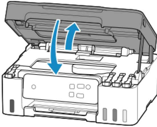
9. Press and hold the **Stop** button and release it when the **Alarm** lamp flashes 9 times.
