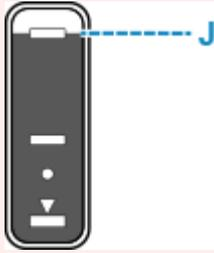
6. Once ink reaches the upper limit line, remove the ink bottle from the inlet.
