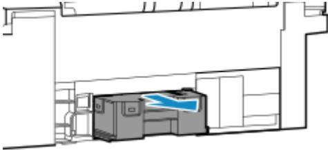
6. Lift the maintenance cartridge a little and pull it out.
