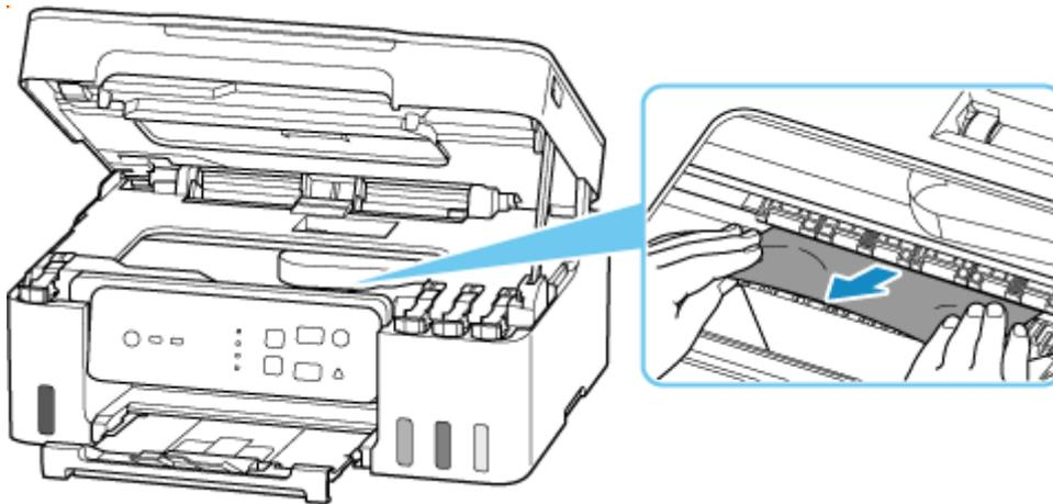
If the paper is rolled up, pull it out and grasp the edges of the paper.
