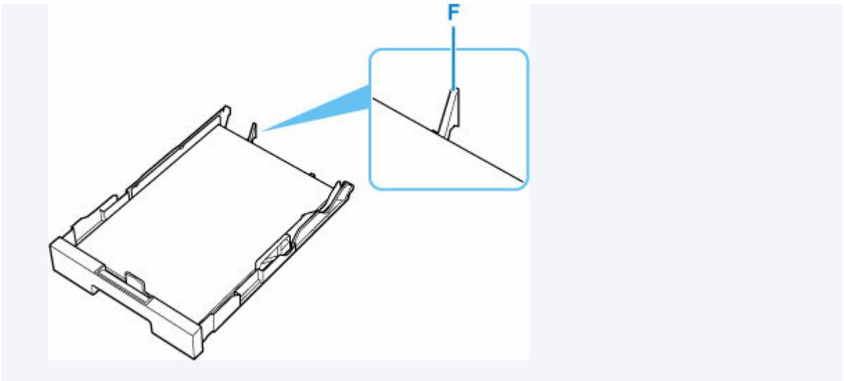
5. Move the front paper guide and adjust the guide to edge of the paper stack.
