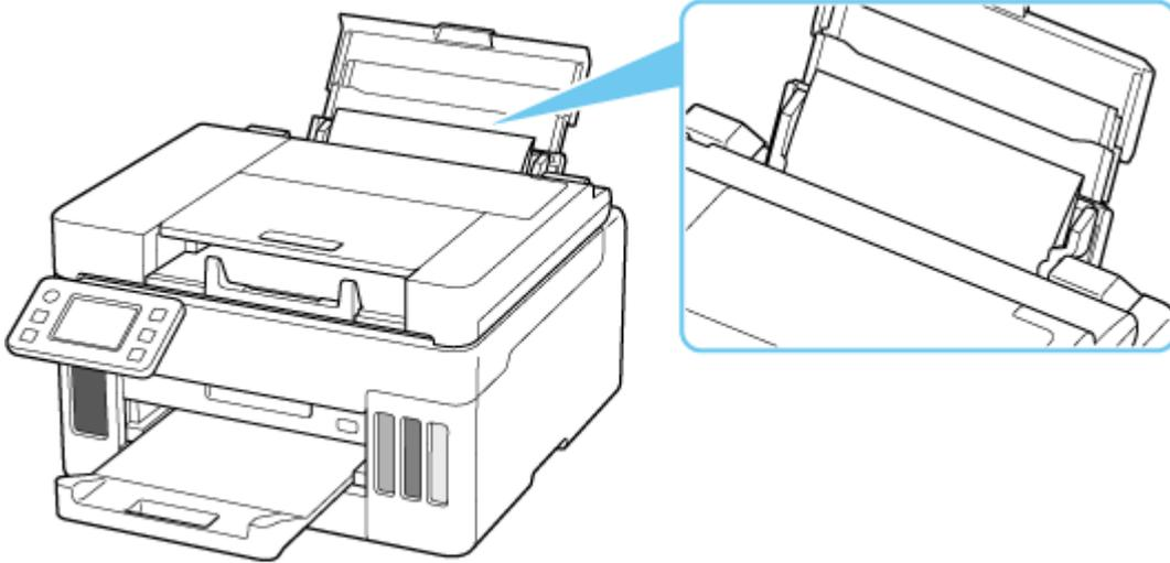
3. Remove foreign object by hand with paper inserted.
