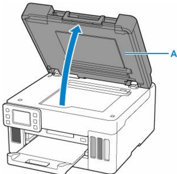
2. Load original WITH THE SIDE TO SCAN FACING DOWN on platen.
