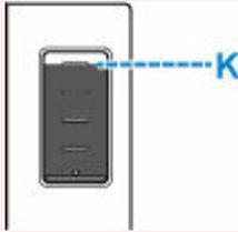
7. Once ink reaches the upper limit line, remove the ink bottle from the inlet.
