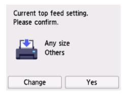
If the paper loaded in the top feed matches the paper information displayed on the printer's touch screen, select **Yes**.
