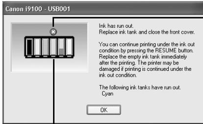
The ink tank with [X] symbol is out of ink. Replace it with a new ink tank.
