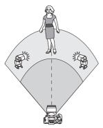
All the slave units will fire at the same output and be controlled to obtain a standard exposure.
