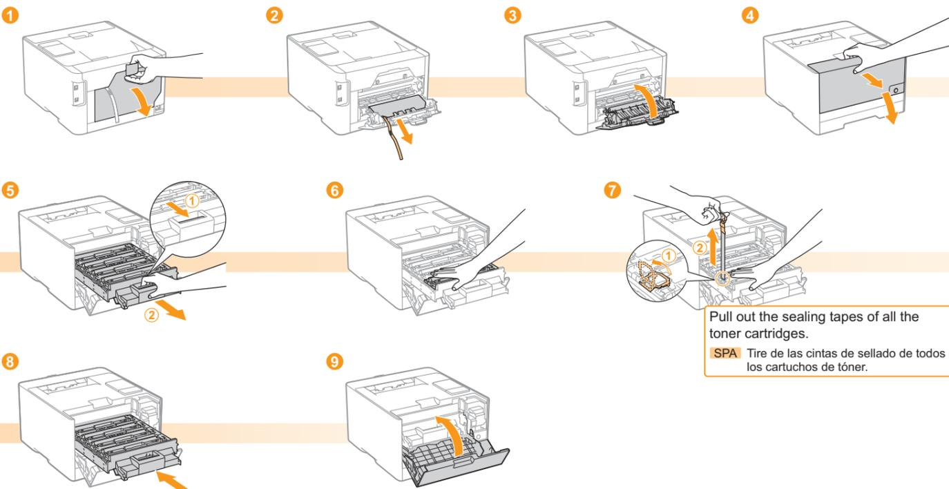
Pull out the sealing tapes of all the toner cartridges.
