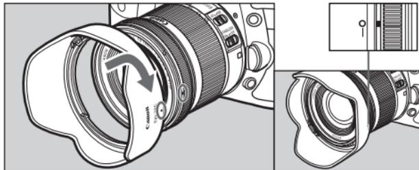
The EW-73C hood cuts out unwanted light and protects the front of the lens from rain, snow, and dust.
