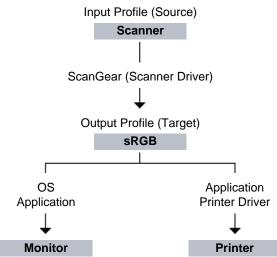
The image's color space is converted from the scanner's color space to sRGB by ScanGear. When displaying on a monitor, the image's color space is converted from sRGB to the monitor's color space based on the operating system's monitor settings and the application's working space settings. When printing, the image's color space is converted from sRGB to the printer's color space based on the application's print settings and the printer driver's settings.
