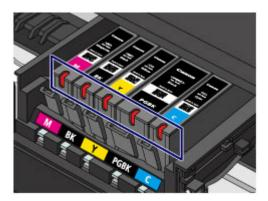
The ink lamp is on. The ink tank is correctly installed.
