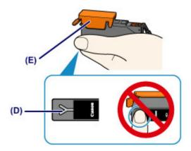
(3) Lift up the tab on the orange protective cap (E) to remove it off GENTLY.
