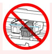
• The printer cannot print unless both the color FINE cartridge and black FINE cartridge are installed. Be sure to install both cartridges.
