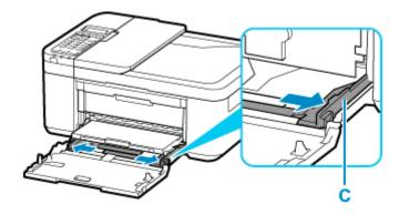
**5.** Load the envelopes in the center of the cassette WITH THE PRINT SIDE FACING DOWN. Fold flap of the envelope and load the envelope in portrait orientation with the address side facing down.
