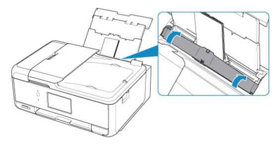
After closing the feed slot cover, the paper setting confirmation screen for the rear tray appears on the touch screen.
