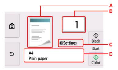
A: The scanning method and copy layout are displayed.
