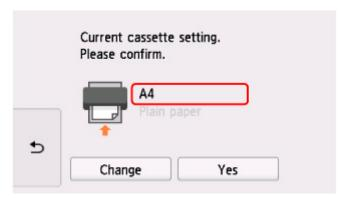
If the page size on the touch screen matches the size of the paper loaded in the cassette, select **Yes**. If not, select **Change** to change the setting in accordance with the size of the loaded paper.
