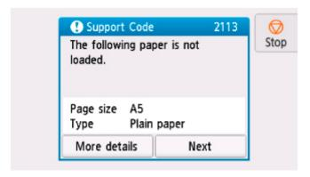
Check the message and select **Next**. When the screen to select the operation is displayed, select one of the operations below.
