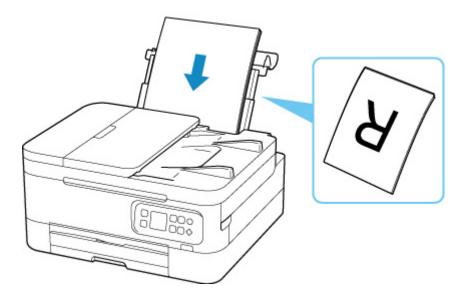
6. Slide right paper guide to align with both sides of paper stack.
