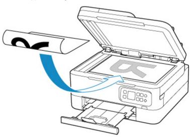
Align the corner of the original with the alignment mark  $\[mathbb{M}\]$ .
