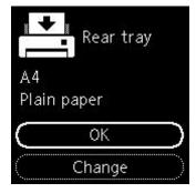
If the page size on the LCD matches the size of the paper loaded in the rear tray, select **OK**. If not, select **Change** to change the setting in accordance with the size of the loaded paper. • When you insert the cassette:
