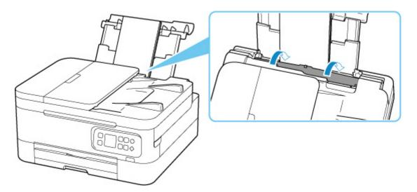
After closing the feed slot cover, the paper setting confirmation screen for the rear tray appears on the LCD.
