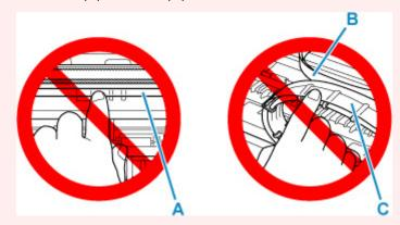
If you soil or scratch this part by touching it with paper or your hand, it could damage the printer.
