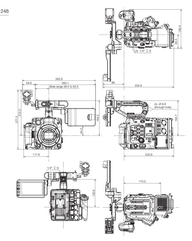
Camera with camera grip, handle unit, microphone holder, LCD monitor (open), LCD attachment unit and optional EU-V3 Expansion Unit 3
