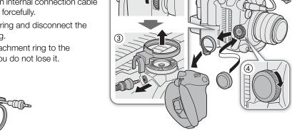
4 Screw the thumb rest onto the camera.
