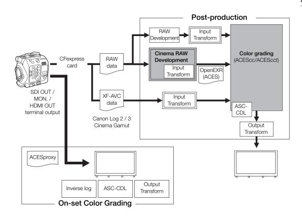
ACESproxy video data that is output from the camera's output terminals when performing
