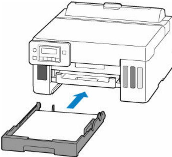
After inserting the cassette into the printer, the paper information registration screen for the cassette appears on the LCD.
