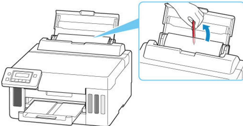
4. Remove the folded paper inserted in step 2.
