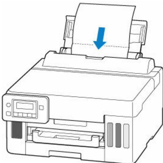
After loading paper on the rear tray, the paper information registration screen for the rear tray appears on the LCD. Select **A4** or **Letter** for **Size:** and **Plain paper** for **Type:**.
