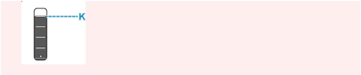
7. Once ink reaches the upper limit line, remove the ink bottle from the inlet.
