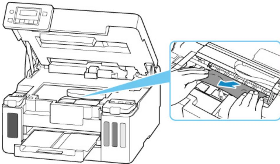
If the paper is rolled up, pull it out and grasp the edges of the paper.
