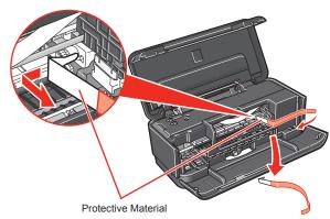
Before turning on the printer, remove all of the shipping tapes.
