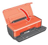
The **Alarm** lamp on the printer still flashes orange if a FINE Cartridge is not installed properly. Open the Top Cover and make sure that position of all the FINE Cartridges is
