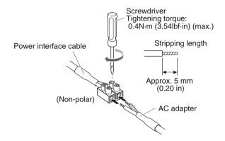
Use a 12-VDC or 24-VAC power supply insulated from 100 VAC.
