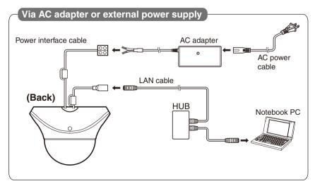
\* The figure shows an example of using an AC adapter (optional) with VB-C500D.
