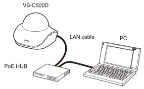
The figure shows an example of connection via a PoE HUB.
