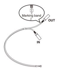
The terminal marked "1" on the marking band (the longer piece from the cable branching point) is used for audio output, while the unmarked terminal (the shorter piece from the cable branching point) is used for audio input.
