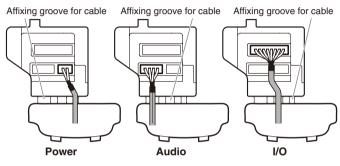
Interface cable fixing method
