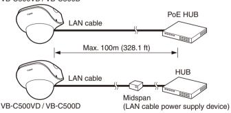
Midspan (LAN-cable power supply) is a device that supplies power to the camera via a LAN cable, just like a PoE HUB.
