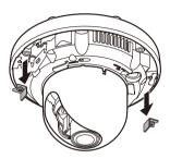
12. Place the dome case on the camera, and affix it by tightening the dome case lock screws.
