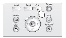
**4.** Press ▲ or ▼ to select **Yes**, and then press the **OK** button. After the roll paper is cut, it is rewound automatically.
