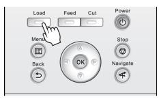
2. Press ▲ or ▼ to select Load Cut Sheet, and then press the OK button.
