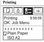
Printing is in progress on the printer. Jobs sent from the computer are printed after the current job. The time left until printing is finished is indicated in the upper-right corner of the screen. (Values exceeding 10 hours are not shown.)
