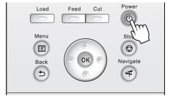
2. The Power Lamp is lit when the printer finishes starting up, and the printer is now in Standby.
