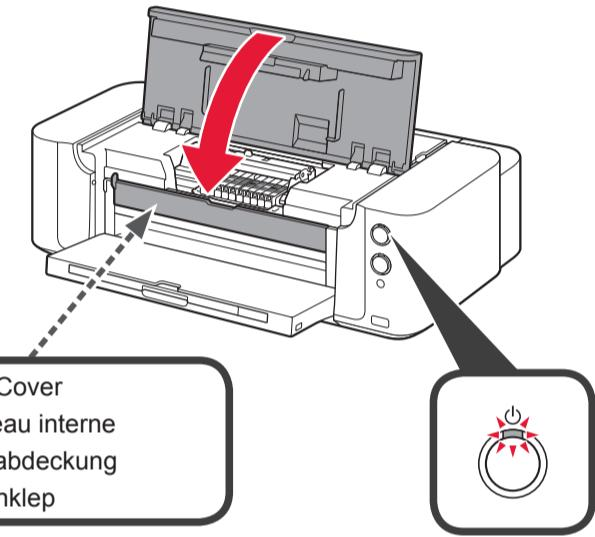
**5** Check that the Inner Cover is closed, then close the Top Cover. Wait for about 3 minutes until the POWER lamp flashes and stays lit white, then proceed.
