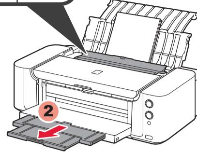
4 Close the Feed Slot Cover, then pull out the Output Tray Extension.
