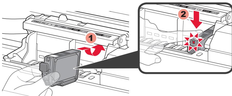
**3** Insert and push down the ink tank into the matching color slot.
