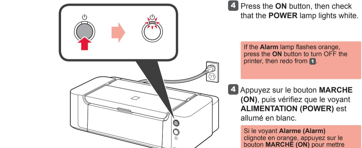
4 Press the ON button, then check that the POWER lamp lights white.
