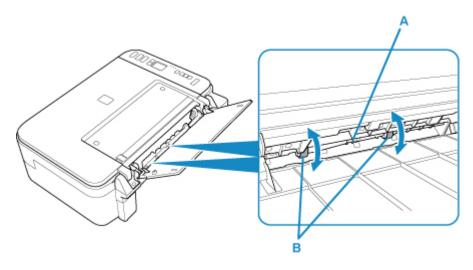
After cleaning the paper feed rollers, turn on the power, then clean the paper feed rollers again.
