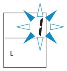
When the segment display changes from flashing to lit, the printer starts copying.
