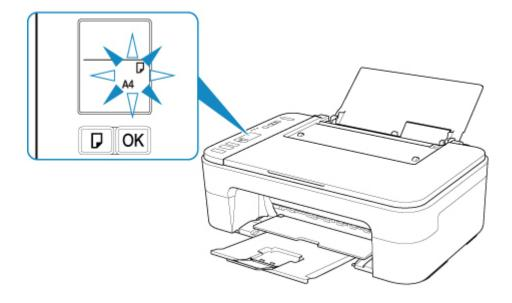
5. Press **Paper Select** button (H) to select a paper size according to the paper loaded on the rear tray and press **OK** button (I).
