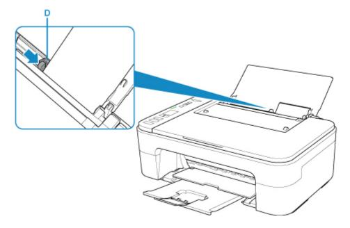
After loading paper on the rear tray, the Paper status and the current paper size flash on the LCD.
