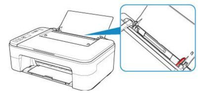
If the paper tears in the rear tray, see List of Support Code for Error (Paper Jams) to remove it.
