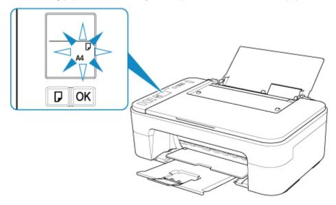
5. Press **Paper Select** button (E) to select a paper size according to the paper loaded on the rear tray and press **OK** button (F).
