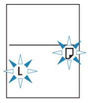
Register the paper size according to the loaded paper.
