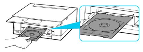
**15.** Insert multi-purpose tray straight in in horizontal direction until arrow (■) on multi-purpose tray guide is approximately aligned with arrow (■) on multi-purpose tray.
