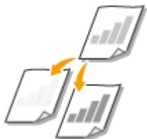
You can adjust the sharpness of the image. Increase the sharpness to sharpen blurred text and lines, or decrease the sharpness to improve the appearance of magazine photos. **Adjusting Sharpness(P. 201)**
