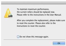
If this message begins to be displayed at startup, purchase an exchange roller kit and replace the worn parts with the consumable parts included in the kit (feed roller and retard roller). See p. 76 for details about the exchange roller kit.
