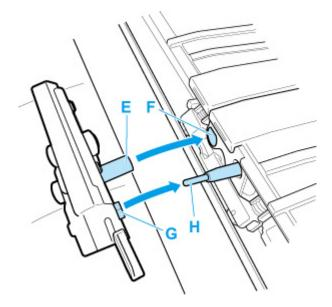
**9.** Install while aligning fixing part included with replacement cutter blade with center of cutter blade.
