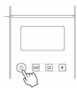
When startup is finished, **ON** button lights up, and printer enters standby mode.
