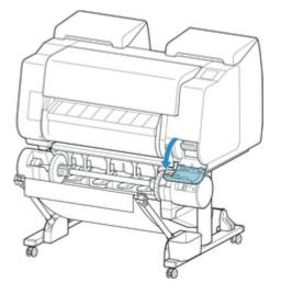
**6.** Hold the used maintenance cartridge by the grip (B) with one hand and put your other hand under the maintenance cartridge to hold it firmly on the bottom, keeping it level as you pull it out.
