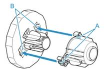
**5.** Insert holder stopper from left into Roll Holder as shown, and while holding in position (B), push firmly until holder stopper flange (A) touches roll paper. Lift holder stopper lever (C) from shaft to lock.
