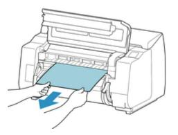
After removing the paper, inspect the interior to ensure paper fragments or other objects do not remain.
