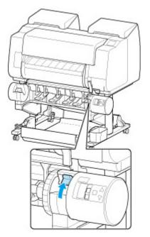
**7.** Hold flanges (A) so that roll holder's black gear is on left, align roll holder shaft with roll holder slot left and right guide grooves (B), and load.
