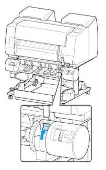
**3.** Hold flanges (A) so that roll holder's black gear is on left, align roll holder shaft with roll holder slot left and right guide grooves (B), and load.
