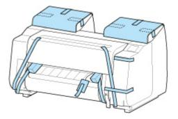
3. If using roll unit, refer to Setup Guide provided with roll unit and attach roll unit to Stand.
