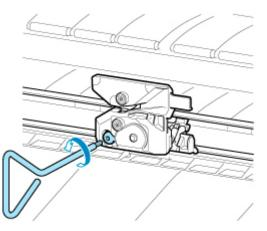
7. Remove cutter blade while holding D.
