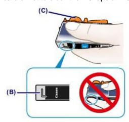
(3) Slowly twist the orange protective cap (C) 90 degrees horizontally to remove it off.
