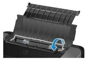
(5) Slide the paper guides (B) to open them, and load the envelopes in the center of the rear tray WITH THE ADDRESS SIDE FACING YOU.
