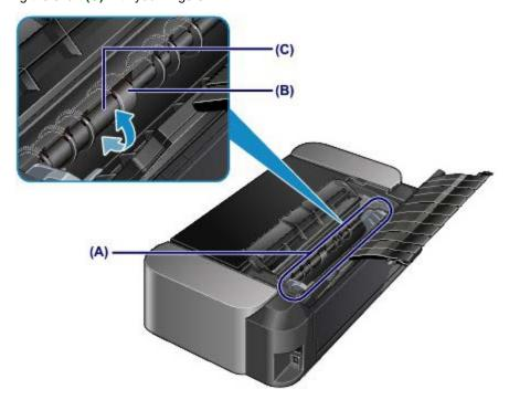
After cleaning the paper feed roller parts with a cotton swab, turn on the power and perform the cleaning from the computer again.
