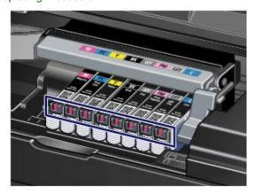
• The ink lamp is on. The ink tank is correctly installed.
