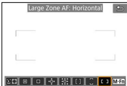
Uses auto selection AF in a horizontal Large Zone AF frame to cover a larger area than Zone AF, which makes focusing easier than with 1-point AF/Expand AF area and also effective for moving subjects.
