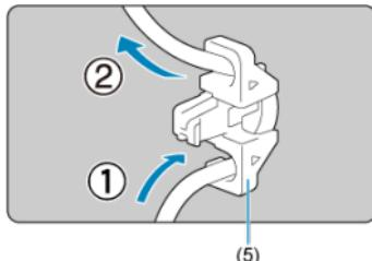
When using an optional Canon interface cable, pass the cable through the clamp (5) as shown before attaching the clamp to the cable protector.
