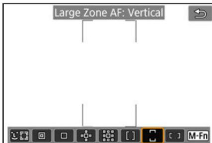
Uses auto selection AF in a vertical Large Zone AF frame to cover a larger area than Zone AF, which makes focusing easier than with 1-point AF/Expand AF area and also effective for moving subjects.
