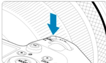
By pressing the < M-Fn > button and turning the < ○ > dial, you can set the ISO speed (1), drive mode (2), AF operation (3), white balance (4), and flash exposure compensation (5).
