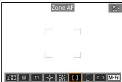
Uses auto selection AF in Zone AF frames to cover a larger area than Expand AF area, which makes focusing easier than with Expand AF area.
