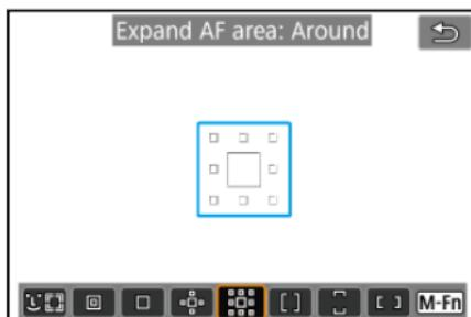
Focuses using one AF point [▪] and surrounding AF points outlined here in blue, which makes it easier to focus on moving subjects than with Expand AF area: ▪▪▪. Servo AF operation is the same as for Expand AF area: ▪▪▪.
