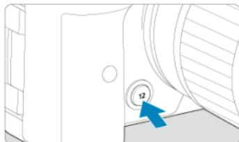
Press the depth-of-field preview button to stop down the lens to the current aperture value setting and check the area in focus (depth of field).
