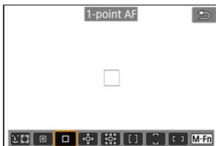
The camera focuses using a single AF point [□].
