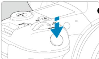
This activates autofocusing and the automatic exposure system that sets the shutter speed and aperture value.
