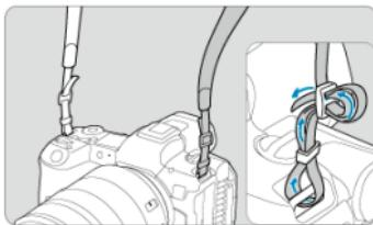
Pass the end of the strap through the strap mount from the bottom, then pass it through the strap buckle as shown. Pull the strap to take up any slack and make sure the strap will not loosen from the buckle.
