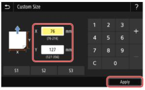
When frequently used non-standard sizes are registered, you can call these up by pressing [S1] to [S3].
