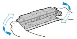
6 Remove the protective cover of the toner cartridge.
