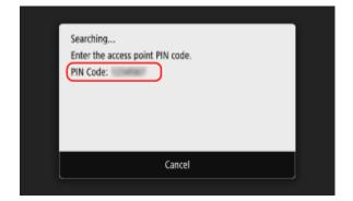
Once this screen is displayed, you must register the WPS PIN code to the wireless LAN router within 10 minutes.
