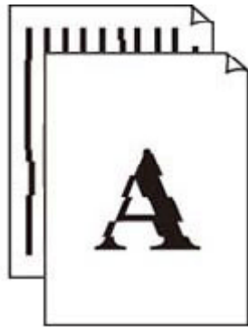
Lines Are Misaligned/Distorted
