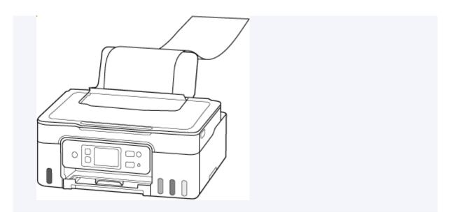
**5.** Move the right paper guide and adjust the guides to both edges of the paper stack. Do not slide the paper guides too tightly against the paper. The paper may not be fed properly.
