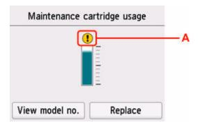
This symbol appears when more than half of the maintenance cartridge has been used. Print head ink refilling and print head replacement operations may be restricted while the symbol is displayed. It is recommended that you prepare a new maintenance cartridge.
