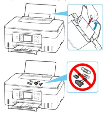
4. Remove the folded paper inserted in step 2.
