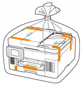
**10.** Attach the protective material to the printer when packing the printer in the box.
