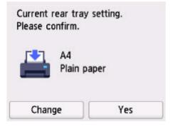
If the page size on the touch screen matches the size of the paper loaded in the rear tray, select **Yes**. If not, select **Change** to change the setting in accordance with the size of the loaded paper. • When you insert the cassette:
