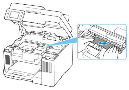
If the paper is rolled up, pull it out and grasp the edges of the paper.
