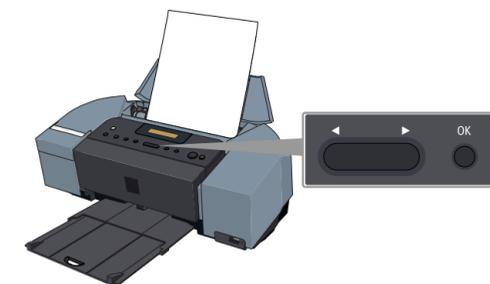
The pattern is printed. And the print head is aligned automatically.
