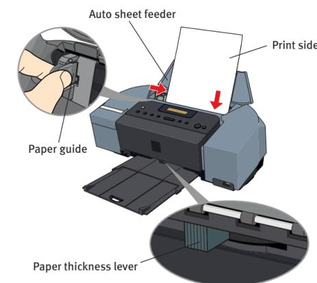
**NOTE:** Ensure that the paper thickness lever is set to the left position.
