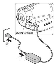
1 Connect the power cord to the compact power adapter.
