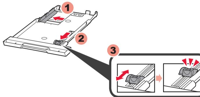
2 Slide the Paper Guide to the sides, then adjust the front guide to the paper size.
