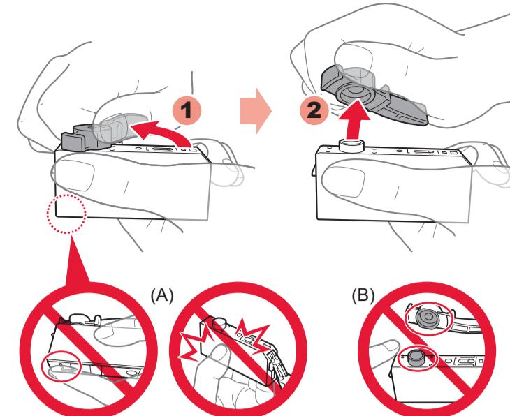
3 Twist and remove the orange cap.
