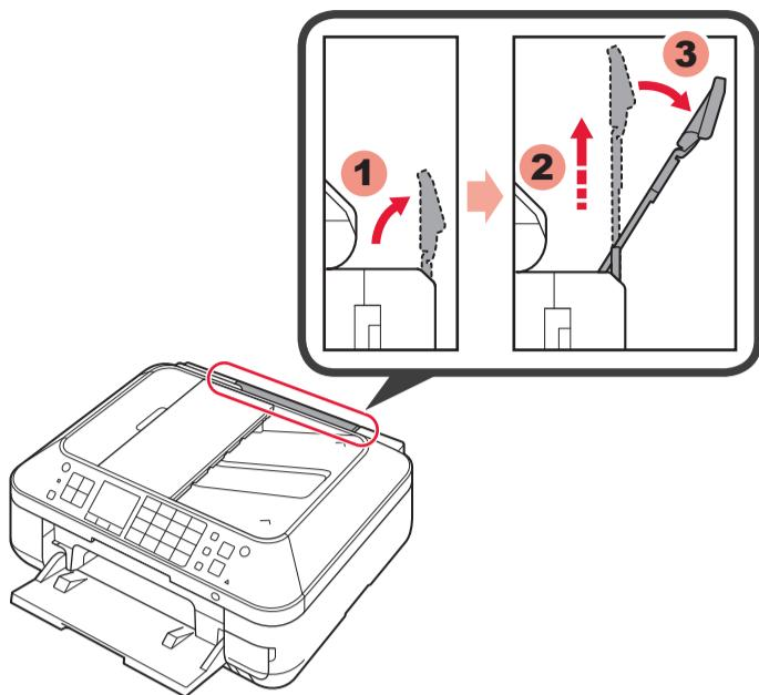
1 Open and extend the Paper Support, then tilt it back in place.
