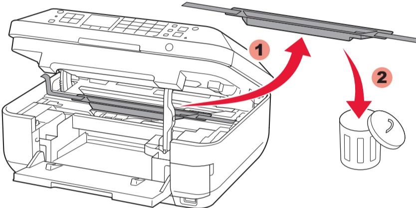
3 Remove the orange tape and protective material.
