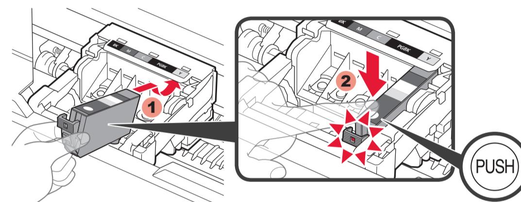
4 Insert and push down the ink tank into the matching color slot.
