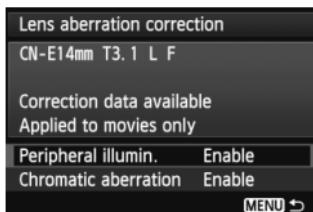
Use EOS Utility (provided software) to register the correction data to the camera. If EOS Utility's correction data registration screen does not show the EF Cinema lens, update EOS Utility to the latest version.
