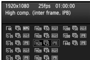
The menu option [**4: Movie rec. size**] enables you to set the movie's image size, frame rate per second, and movie recording/compression method. The frame rate switches automatically depending on the [**3: Video system**] setting.
