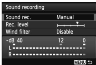
You can shoot movies while recording sound with the built-in monaural microphone, with a commercially-available stereo microphone, or with Line input. You can also freely adjust the sound-recording level.
