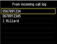
Use the ▲▼ button to select a fax/telephone number or a name, then press the **OK** button.
