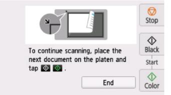
If you continue scanning, load the original on the platen glass and start scanning.
