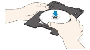
12. Insert the disc tray into the disc tray guide.
