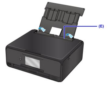
After closing the feed slot cover, the paper information registration screen for the rear tray is displayed on the LCD.
