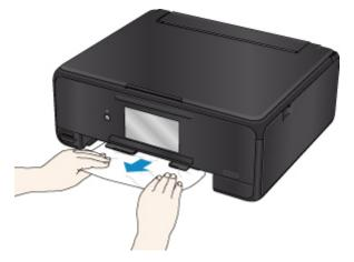
If the measures above do not solve the problem, see <u>Removing Jammed Paper from Rear Side</u> to open the rear cover and to remove the paper.
